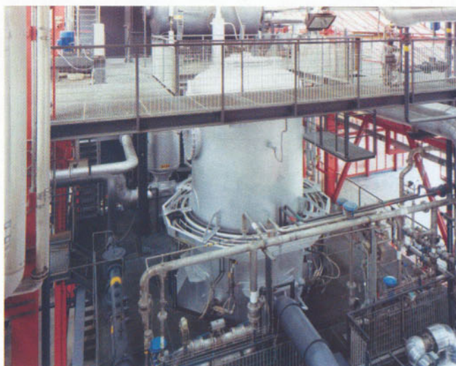
The process simultaneously gasifies organic waste fractions and melts down inert materials
